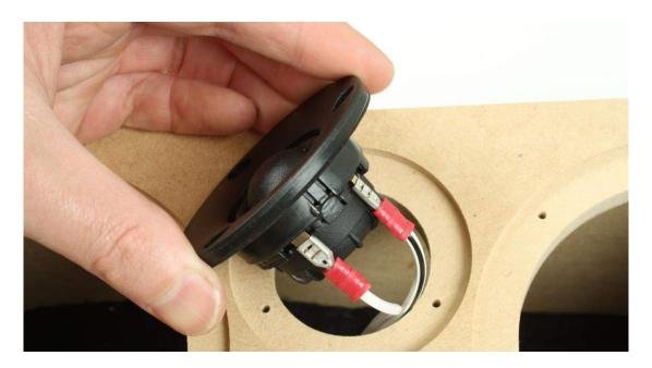
If you find they are too tight, avoid undue force that could damage the tweeter terminals. Instead, use a small flat head screw driver to gently prize open the spade connector. This is shown over the page.
