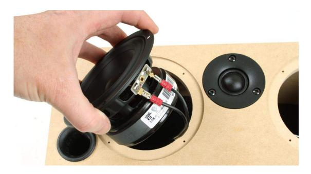
Lower the woofer gently into the hole and angle the driver so that the terminals are clear of the cut out on the way down.
