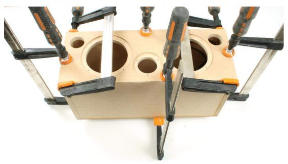
Before clamping, make sure each edge is carefully aligned - a little care here will ensure the best result. Once you have clamped the box, ensure you wipe off any excess glue that has been squeezed out. Once the glue has dried remove the clamps. To obtain a smooth finish, lightly sand the edges of the panels with a fine grade sandpaper, about 180 grit works best. If you plan to paint or varnish the box a little extra effort now to remove all traces of glue and rough edges will be well worth it.
