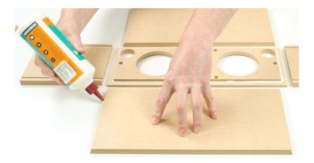
Apply glue to the edge of the top and bottom panels as shown above. Now assemble the side and top panels, aligning the rail on the edge of the top with the trench in the side panel, as shown below.
