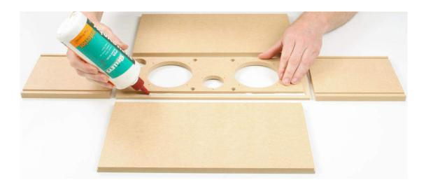
Lay out the side panels as shown. Apply glue to the trench around the perimeter of the front baffle. Apply glue also to the trench of the side panels as shown below.
