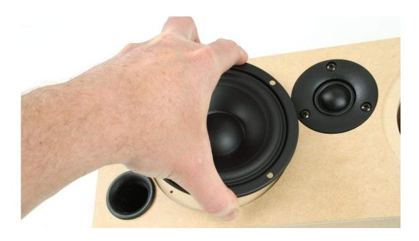
Fix the woofers into place. Note how the screw driver is braced with the other hand.
