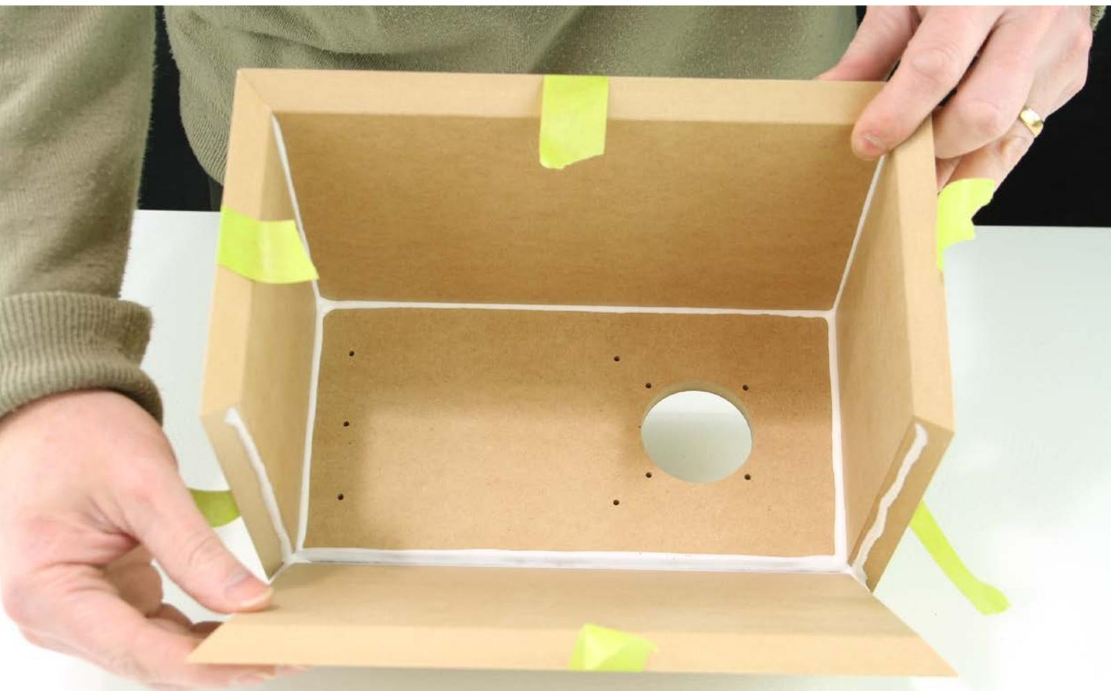
Apply a single thick bead for the top and side panels. Test the first pair of mitres to confirm glue coverage, then glue and fold up all the other panels. It is best to fold up and then tape one join at a time. Ensure the glue covers the joint before moving on to the next step.
