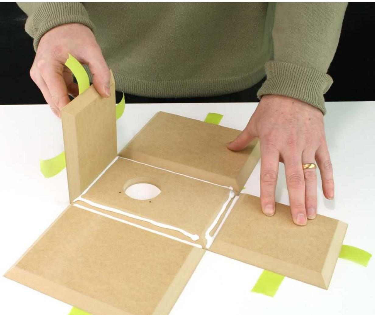
Confirm the amount of glue applied by folding up the first panel. The glue should cover the entire surface in contact. It's preferable to see the glue ooze beyond the joint slightly. This provides visual feedback on whether the glue has set. Once set, PVA glue becomes transparent.
