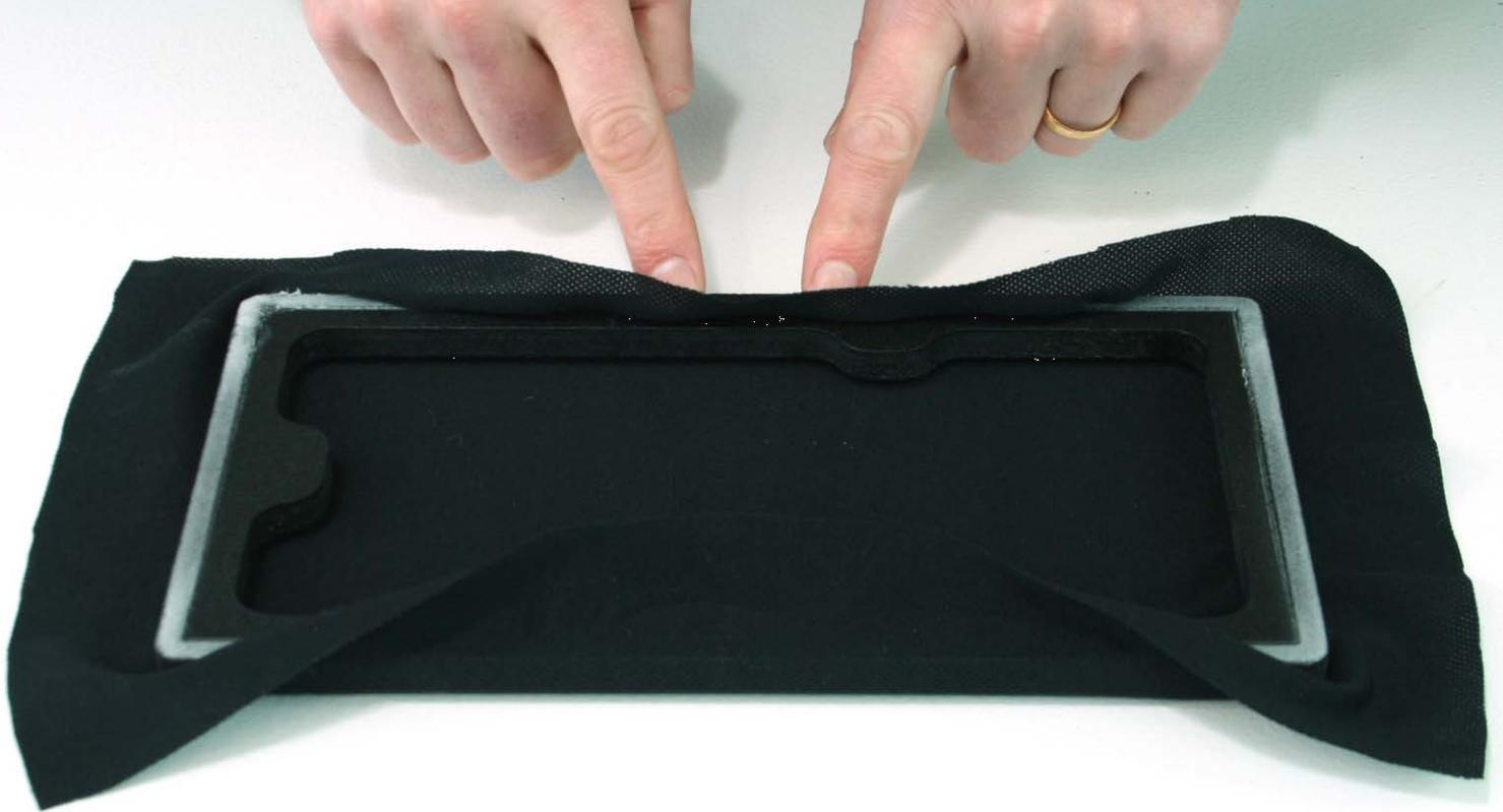
Now press the cloth onto the glue on the back of the frame. Start with one side but avoid the corners, which should be pressed on last. It's critical that the corners are done as the final step to avoid wrinkles bunching up. Next press the cloth onto the opposite edge. You may notice wrinkles appearing. This is an indication that sufficient tension has been applied.
