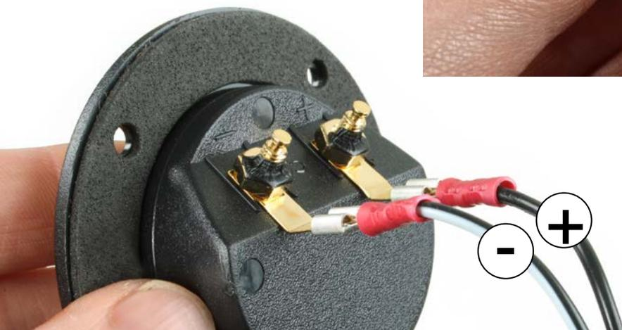
**Note:** The cable with the white strip goes to the negative terminal
