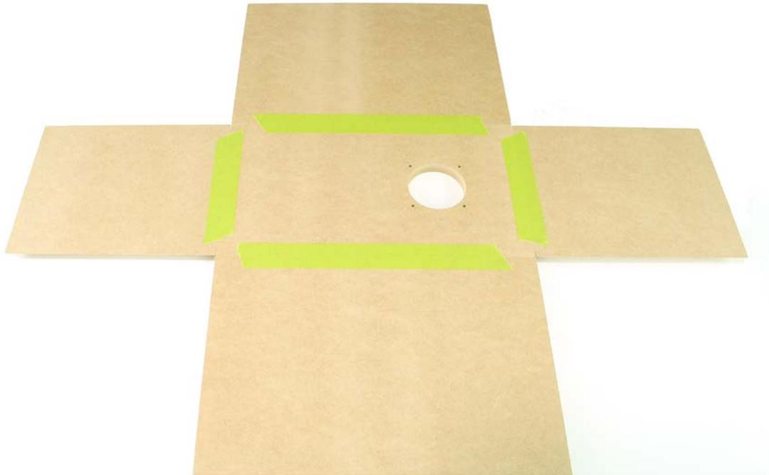
Tape all four joints where the rear panel meets the side and top panels. It's a good idea to avoid covering the corners so that you can ensure all panels remain aligned during taping.
