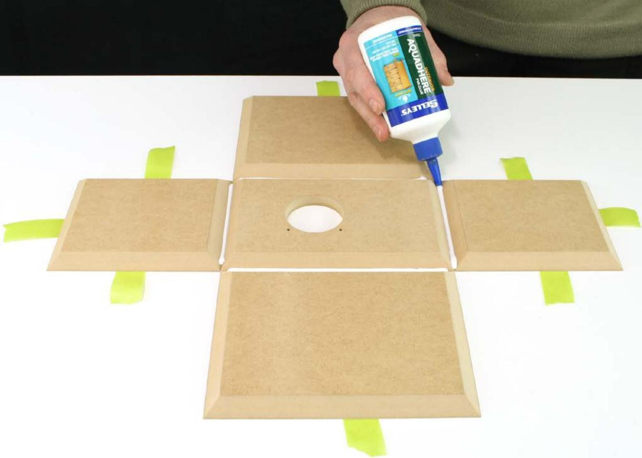
**Tip:** placing masking tape as shown assists with folding up the panels.
