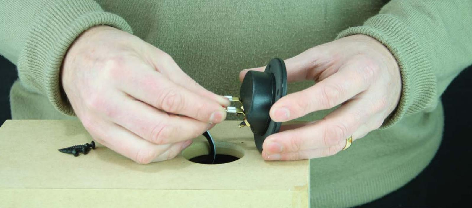
We recommend using a Phillips head screwdriver, as some powered drivers are more likely to cause damage if the head slips off the screw head. Impact drivers should be avoided. If using a powered driver, it's best to use one which has a clutch, so that once the screws are adequately tightened, the driver will not over-tighten. This avoids stripping the MDF pre drilled holes or damage to the screw heads. If using a screwdriver, your left hand can hold the shaft to avoid slipping.
