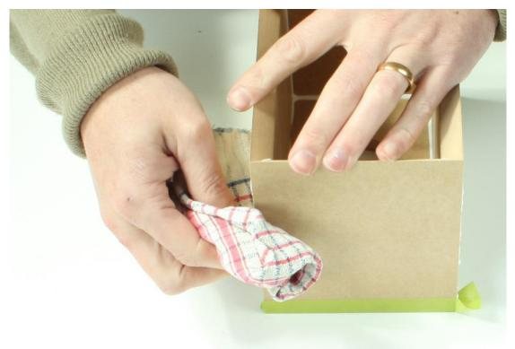
Apply a thick glue bead around the internal surfaces of the miters. You may prefer a zig zag pattern with a thinner bead. It's a good idea to remove the panel and confirm even coverage.
