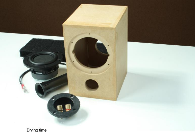
Typical wood glues can achieve moderate strength in as little as 30 minutes. If you are using PVA glue then a good indicator that it has set is the transparency. PVA becomes transparent once set. Ideally it's best to leave the enclosure clamped over night before moving on to assembly or finishing.
