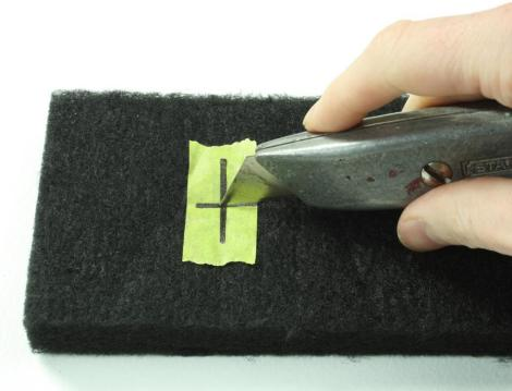
Insert the lining, feeding the cable through the cross shaped cut out.
