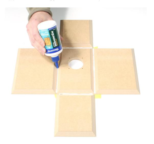
Apply a second bead. Since the glue will tend to run down towards the bottom, it's a good idea to apply the glue above half way up to ensure even coverage.
