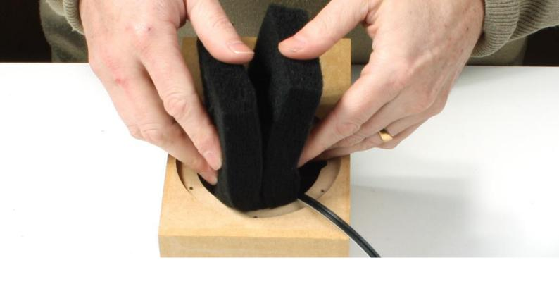
Before inserting the acoustic lining, cut an opening in the shape of a cross with a sharp blade. The cross should be centered 205mm from the top end.
