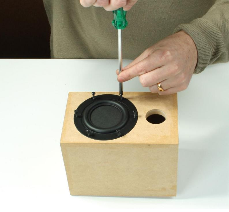
Screw the driver into place with a Phillips head screwdriver, securing the shaft with the other hand. Pushing the port into place completes the assembly. Your new kit is now ready to rock!
