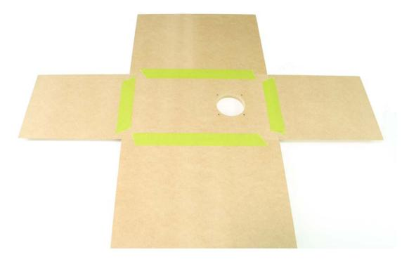
Tape all four joints where the rear panel meets the side and top panels. It's a good idea to avoid covering the corners so that you can ensure all panels remain aligned during taping.
