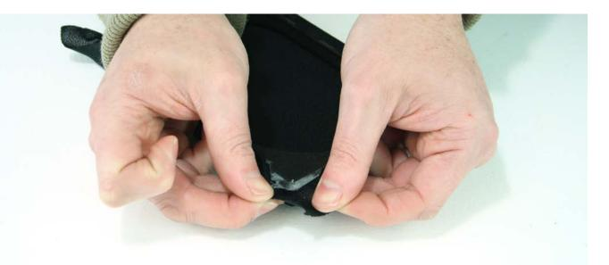
Hold the cloth with both hands, then pull it back over the frame. Stretch it firmly, pulling back into the correct position. After stretching it into place, press down to the glue area.
