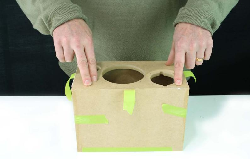
Once you have confirmed adequate glue coverage, press the baffle into place and wipe off all excess glue with a damp cloth. Secure panels firmly with masking tape. Apply pressure when pressing the tape into position. The tape holds the panels together as the glue sets.
