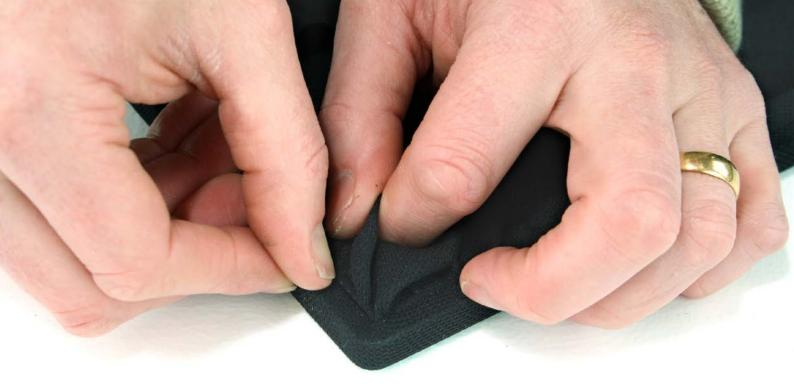
Now you can use your thumbnail to find the cut line. Pressing your nail into the trench, score all the way around. Then with a sharp blade, slowly and carefully cut away the grille cloth, using the trench as a guide.
