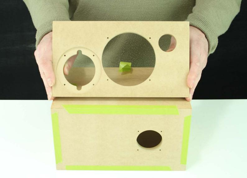
Ensure the front baffle has the correct orientation. The port on the front and terminals on the back should be oriented so they are both on the bottom. In the picture above they are both on the right as the speaker is placed on its side.
