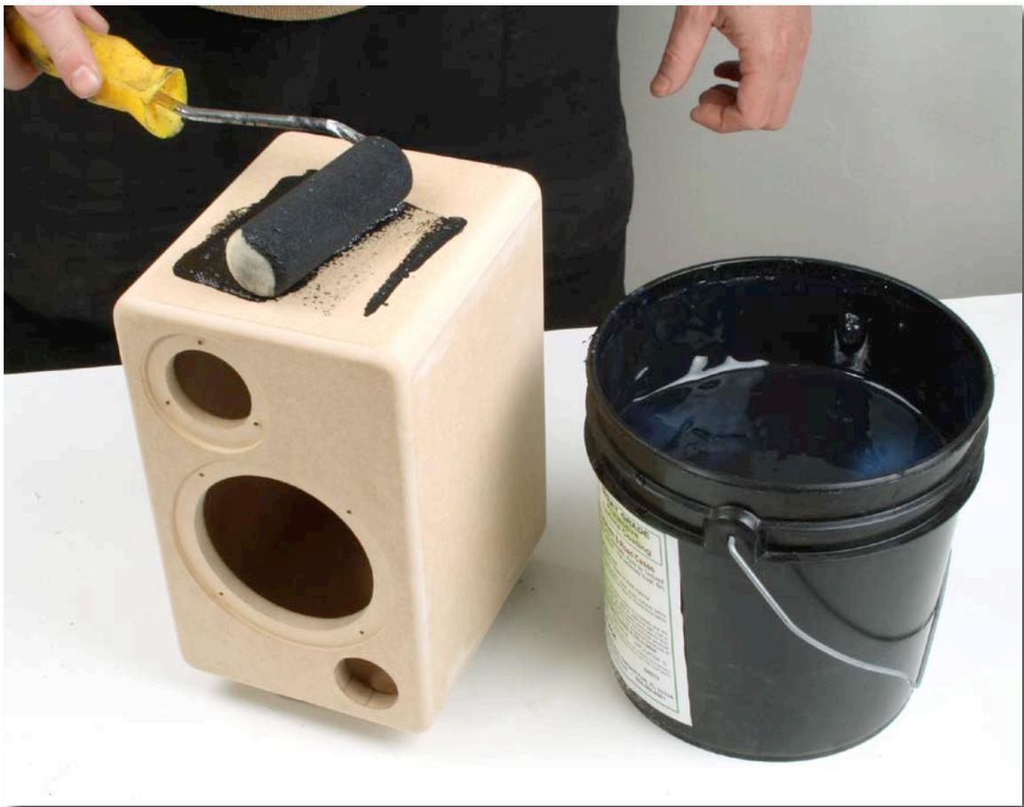
Be careful in applying the coat to the front baffle (image 8). This coat should be quite thin, otherwise the paint will get into the driver recesses which potentially means the drivers won't fit.
