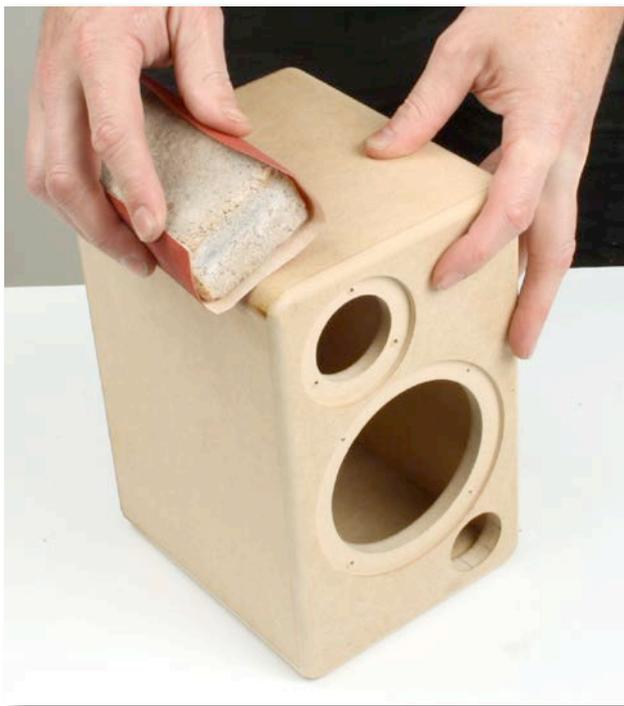
If you are completing this optional step, you will also need to do another round of filling. The rounding process will take off a lot of the original filler and will sometimes expose voids where the filler wasn't pushed down far enough in the first step.
