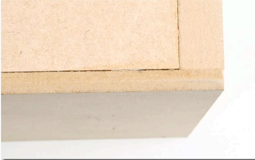
As you can see in the photo above, gaps in the joints can also be present due to inadequate pressure during the construction process. These should also be filled using a spackle filler. Please note that many fillers are not suitable for use with DuraTex. Be sure to use a spackle type filler (shown below). Make sure you also observe the drying times on the filler you are using before proceeding.
